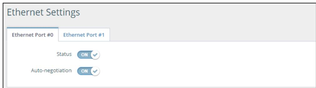
**Ethernet Port#1 Settings** Ethernet Port#1 only supports the Status switch to enable or disable the port.
